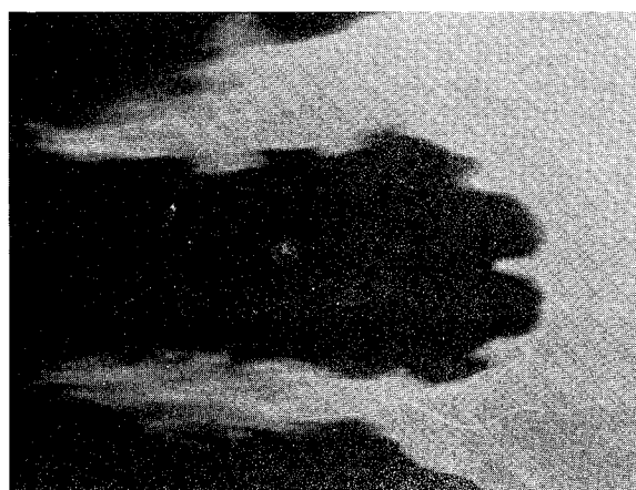
Fig. 5 Breakup of a waterdrop in a shock tube; final stage.
